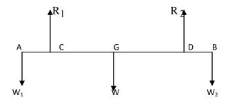
There is upward reaction  $R_1$  at C.
