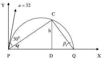
Given, initial velocity u = 32 m/sec,  $30^0$  is the angle of projection. P-be the point of projection. 't' – be the time taken from P to C.
