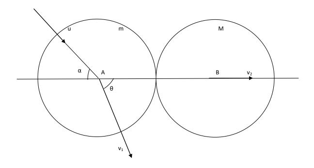
Considering the sphere M, its tangential velocity before impact is zero and hence after impact also, its tangential velocity is zero.
