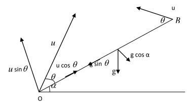
Let u be the given velocity of projection and  $\theta$  the inclination of the direction of projection with the plane. u has two components  $u\cos\theta$  along the upward inclined plane and  $u\sin\theta$ perpendicular to the inclined plane. g has two components, g sin  $\alpha$  along the downward inclined plane and gcos  $\alpha$  perpendicular to the inclined plane and downwards.
