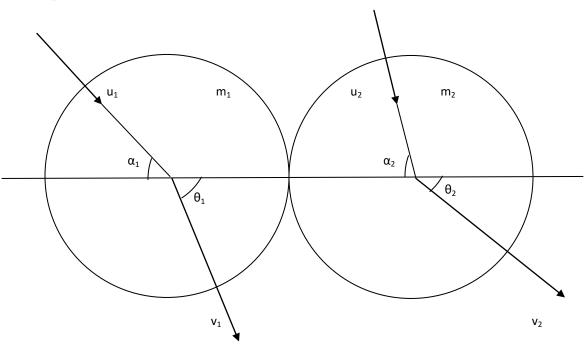
Let the velocities of the spheres after impact be  $v_1$  and  $v_2$  in directions inclined at angles  $\theta_1$  and  $\theta_2$  respectively to the line of centres. Since the spheres are smooth, there is no force perpendicular to the line of centres and therefore, for each sphere the velocities in the tangential direction are not affected by impact.
