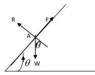
Let  $\theta$  - be the inclination of the rough inclined plane, on which a particle of weight W, is placed at A. Forces acting on the particle are,
