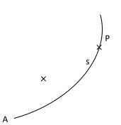
If P is the position of a particle on a curve at time t and if the tangential acceleration at P varies as the arcual distance of P measured from a fixed point A on the curve and is directed towards A, then the motion of P is said to be simple harmonic.
