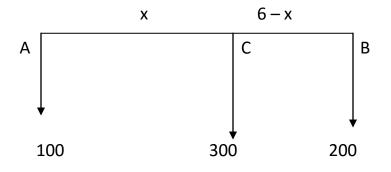
Let A be the weaker man bearing 100 kgs., B the stronger man bearing 200 kgs. Let C be the point on AB where the stone is fastened to the pole, such that AC = x. Then the weight of the stone acting at C is the resultant of the parallel forces 100 and 200 at A and B respectively. 100 AC = 200 BC
