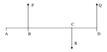
P, Q, R are parallel forces acting on the rod AD at B, D, C respectively.
