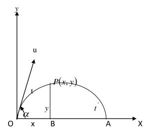
Let u be the velocity of projection,  $\alpha$  be the angle of projection, P be the position of the particle after t secs. Let t' be the time taken to travel from P to A
