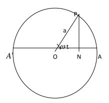
Let AA' be the diameter of the circle with centre O and P be the position of the particle at time  $t \sec s$ . Let N be the foot of the perpendicular drawn from P on the diameter AA'. P moves along the circumference of the circle with uniform speed and describes equal arcs in equal times. Let  $\omega$  – be the angular velocity.  $\therefore \angle AOP = \omega t$
