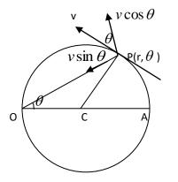
Let O – be the fixed point (pole), OC – initial line. Polar equation of the circle is  $r = 2 a \cos \theta$ . Let P (r,  $\theta$ ) be the position at time't' Angular velocity about O is  $\dot{\theta} = w$ (constant)
