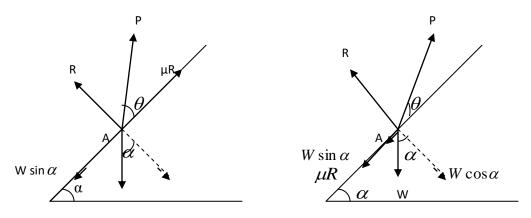
Let  $\alpha$  be the inclination of the plane, W be the weight of the body, P – be the force acting at an angle  $\theta$  with the inclined plane and R – be the normal reaction.
