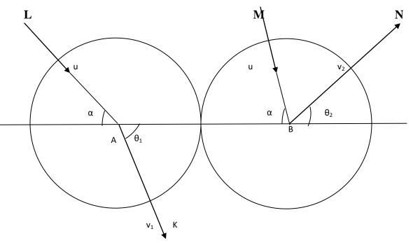
Let m be the mass of either sphere: AB is the line of impact. Before impact, the directions of motion are LA and BM making the same acute angle  $\alpha$  with AB as shown in the figure. Let u be their velocity.
