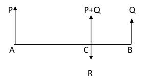
Let P, Q, R be the three coplanar parallel forces in equilibrium. Draw a line to meet the forces P, Q, R at the points A, B, C respectively.
