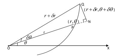
Consider a particle moves in a plane curve. Let P (r,  $\theta$ ) be its position in time t and  $Q(r + \delta r, \theta + \delta \theta)$  be its position in time t+ $\delta$  t. Take O – as the pole and OX- as initial line. Velocity along the radius vector OP in the direction of r increasing is called the radial velocity and the velocity in the direction  $\perp$  r to OP in the direction of  $\theta$  increasing is called the transverse velocity.
