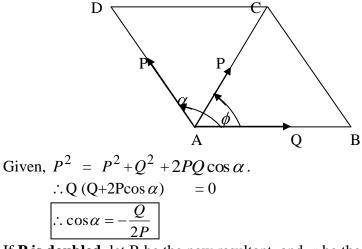
If **P** is doubled, let R be the new resultant, and  $\varphi$  be the angle between Q and R.
