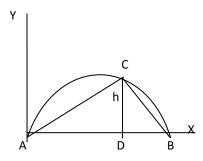
Let u be the velocity of projection and  $\alpha$  the angle of projection and let t secs be the time taken from A to C. Draw CD  $\perp$  AB and let CD = h.
