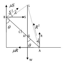
Forces are acting as marked in the figure. For equilibrium, the three forces R', S', W must be concurrent at L, where W – be the weight of the ladder.
