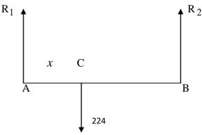
AB is the light pole of length 8m. C is the point from which the load of 224 kgs. is hung. Let AC = x. Then BC = 8 - x. given (8 - x) - x = 2i.e) 8 - 2x = 2 Or 2x = 6.  $\therefore x = 3$ . i.e. AC = 3 and BC = 5.
