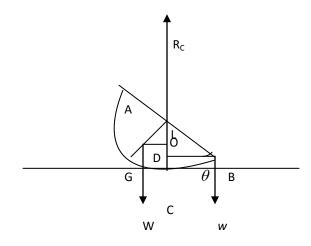
Draw GL perpendicular to OC and BD perpendicular to OC. Base AB is inclined at an angle  $\theta$  with the horizontal BD. Forces acting are i) Reaction R<sub>c</sub> ii) Weight W at G iii) Weight w at B.
