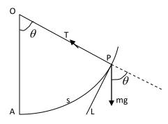
Let OA = l be the length of the pendulum where O is the point of suspension. Let 'm' be the mass of the bob and P be the position of the bob in time t secs and arc AP = s,  $AOP = \theta$ The two forces acting are i) mg( $\downarrow$ ) ii) Tension T along PO. mg is resolved into two components i) mg cos  $\theta$  along OP. ii) mg sin  $\theta$  along PL. mg  $\cos \theta$  and T balances each other.
