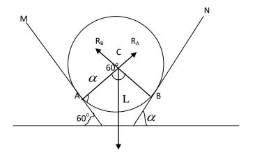
Let the sphere centre C rest on the inclined planes AM and BN. MA makes  $60^{\circ}$  with the horizontal and let NB make an angle  $\alpha$  with the horizon.
