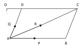
Through O, draw a line parallel to the direction of P, to meet the line of action of Q at D. Complete the parallelogram ABCD such that AB, AD represent the magnitude of P and Q and the diagonal AC represents the resultant R of P and Q.
