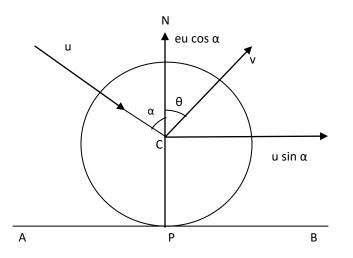
Let AB be the plane and P the point at which the sphere strikes it. The common normal at P is the vertical line at P passing through the centre of the sphere. Let it be PC. This is the line of impact. Let the velocity of the sphere before impact be u at an angle  $\alpha$  with CP and v its velocity after impact at an angle  $\theta$  with CN as shown in the figure.
