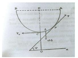
Let ACB be a uniform heavy flexible cord attached to two points A and B at the same level, C being the lowest, of the cord. Draw CO vertical, OX horizontal and take OX as X axis and OC as Y axis. Let P be any point of the string so that the length of the are CP = s
