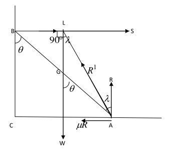
Since the wall is smooth, there is no frictional force. Forces acting on the ladder are i) its weight W, ii) Frictional force  $\mu R$  iii) R at A iv) S at B. For equilibrium, the three forces W, R', S must be concurrent at L. where  $R^1$  is the resultant of R and  $\mu R$ . In triangle LAB,
