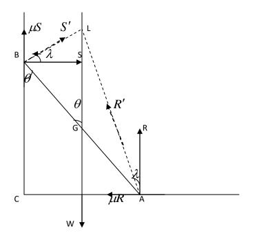
When the ladder AB is in limiting equilibrium, five forces are acting as marked in the figure.
