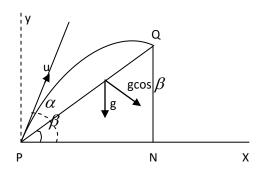
Let P be the point of projection on a plane of inclination  $\beta$ , u be the velocity of projection at an angle  $\alpha$  with the horizontal. The particle strikes the inclined plane at Q. Then PQ = r is the range on the inclined plane. Take PX and PY as x and y axes.
