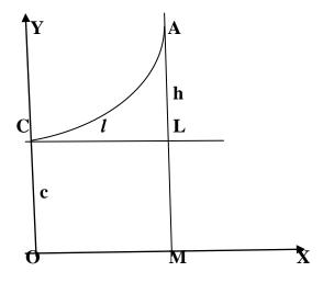
C is the vertex of the catenary CA, A being the kite. The origin O is taken at a depth c below C.
