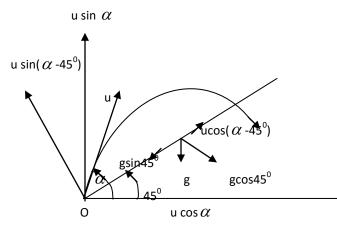
When the particle strikes the plane at right angles, velocity parallel to the plane is zero.
