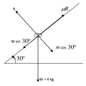
Since the body is in limiting equilibrium on the inclined plane, it tries to move in the downward direction along the inclined plane.
