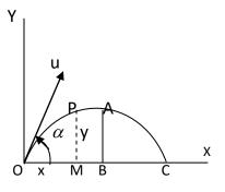
Let a particle be projected from O, with initial velocity u and  $\alpha$  be the angle of projection. Take OX and OY as x and y axes respectively. Let P (x,y) be the position of the particle in time t secs. Now u can be divided into two components as  $u \cos \alpha$  in the horizontal direction and  $u \sin \alpha$  in the vertical direction. Now, horizontal velocity  $u \cos \alpha$  is constant throughout the motion.
