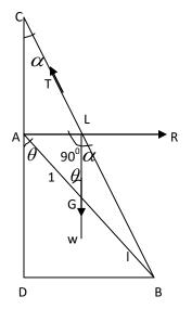
AB is the rod of length a, with G its centre of gravity and BC is the string of length *l*. The forces acting on the rod are:
