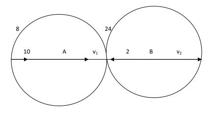
Let  $v_1$  and  $v_2$  cm/sec. be the velocities of the 8gms and 24 gms mass respectively after impact.
