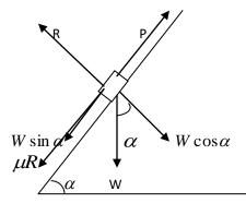
Let P be the external force applied to keep the body at rest. Resolving the force,
