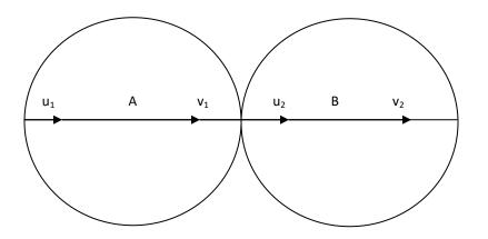
AB is the line of impact, i.e. the common normal. Due to the impact there is no tangential force and hence, for either sphere the velocity along the tangent is not altered by impact. But before impact, the spheres had been moving only along the line AB (as this is a case of direct impact). Hence for either sphere tangential velocity after impact = its tangent velocity before impact = 0. So, after impact, the spheres will move only in the direction AB. Let their velocities be  $v_1$  and  $v_2$ .
