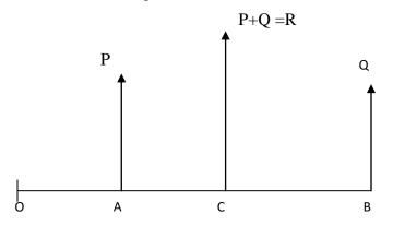
Let P and Q be the two parallel forces acting at A and B. P + Q be their resultant R acting at C. such that
