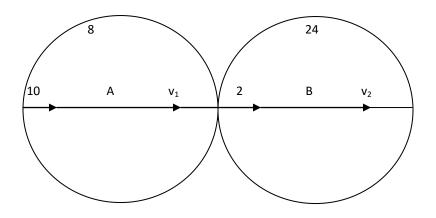
Let  $v_1$  and  $v_2$  cm. per sec. be the velocities of the masses 8gm and 24 gm respectively after impact.
