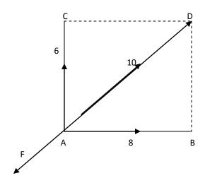
Let AB = 8 and AC = 6 represent the directions of the forces, A being the particle.
