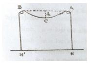
The tension of the chain is unaltered by passing overt the smooth peg A. The tension at A can be calculated by two methods.
