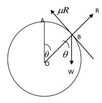
Let O be the centre, A the highest point of the sphere and B the position of the particle which is just on the point of motion. Let  $\angle AOB = \theta$
