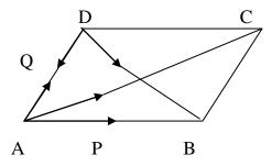
Let the forces P and Q acting at A be represented in magnitude and direction by the lines AB and AD. Complete the parallelogram BAD.
